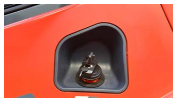
The oil filler is equipped with a lock, which is safe and reliable.
