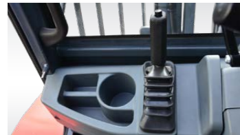
Ratchet type hand brake is reliable and has low operating force.
